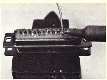
Photo 4. Insert the wire into the connector. Avoid excessive and prolonged heat to prevent damage to the connector.
